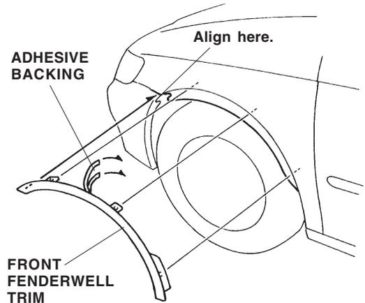
5. Align the fenderwell trim with the front bumper as indicated by the arrow. While holding light pressure against the fenderwell trim over the inner fender liner, slowly and carefully remove the lower adhesive backing you peeled back. Next, remove the upper adhesive backing the same way.
