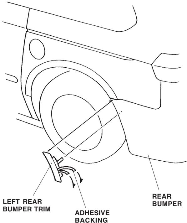
17. Align the bumper trim with the rear bumper as indicated by the arrow. While holding light pressure against the bumper trim, slowly and carefully remove the lower adhesive backing you peeled back. Next, remove the upper adhesive backing the same way.
