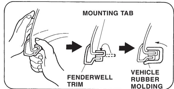
14. Reinstall the vehicle rubber molding around the fenderwell over the mounting tabs.
