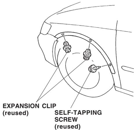
8. Turn the steering wheel all the way clockwise, and repeat steps 2 through 7 to install the right front fenderwell trim.
