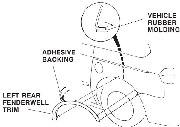
11. Align the fenderwell trim with the rear bumper as indicated by the arrow. While holding light pressure against the fenderwell trim, slowly and carefully remove the lower adhesive backing you peeled back. Next, remove the upper adhesive backing the same way.
