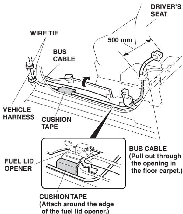
13. Using isopropyl alcohol on a shop towel, thoroughly clean the edge of the fuel lid opener where the cushion tape will attach. Remove the adhesive backing from one cushion tape, and attach it to the edge of the fuel lid opener as shown.
