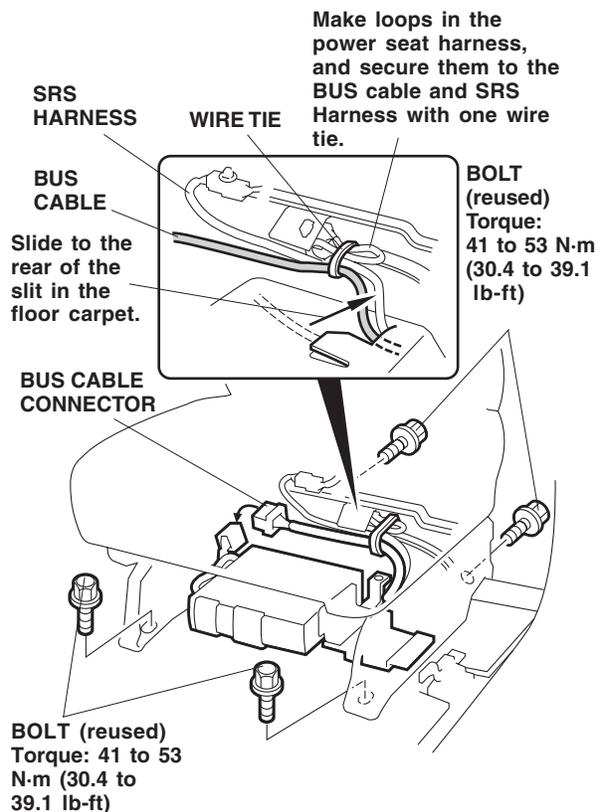
28. Check that all wire harnesses are routed properly and all connectors are plugged in.
