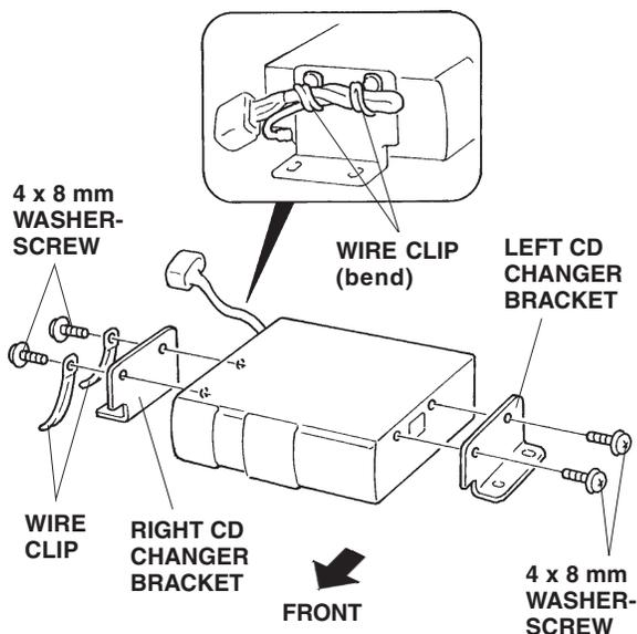
24. Bundle the excess BUS cable, and secure it to the CD changer with the two wire clips.
