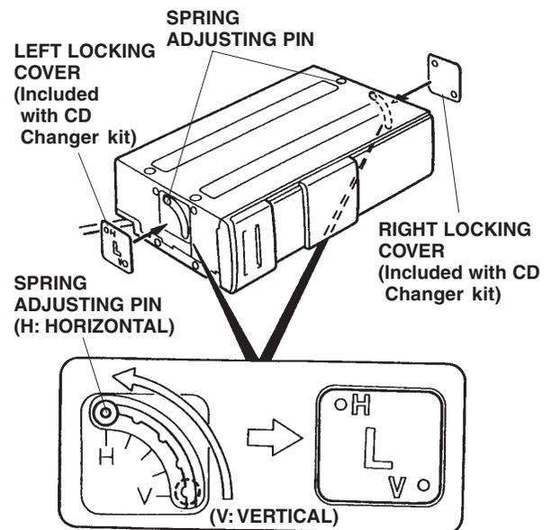
22. Remove the adhesive backing from the "L" and "R" locking covers, and attach them to the sides of the CD changer. Align the diagonally opposite holes with the H and V positions.
