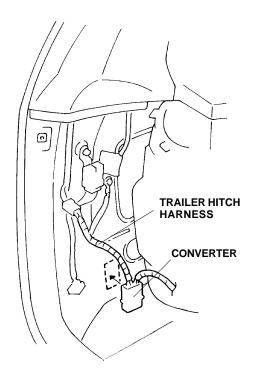
19. Secure the trailer hitch harness to the vehicle harness with one small wire tie; then secure the harness to the body with one cushion tape in the area shown.
