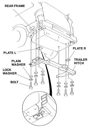
Torque the trailer hitch bolts to 79 N•m (7.9 kgm, 58 lb-ft). 10. Remove the tailgate weatherstrip and rear panel (ten clips and two self-tapping screws).
