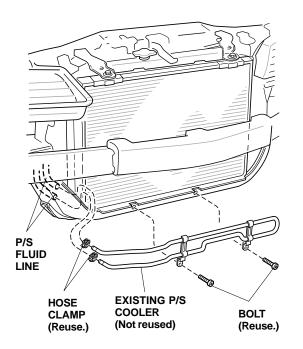
31. Place the heavy-duty P/S cooler on the radiator bulkhead, attach the P/S lines with the hose clamps, and reinstall the two bolts removed in step 30. Tighten the hose clamps and the center bolt, then remove the outboard bolt.
