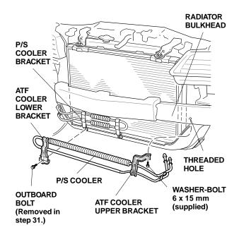
33. Remove the ATF return line from the radiator return pipe, and attach it to the lower ATF cooler pipe using one new hose clamp from the kit.
