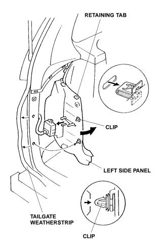
14. Remove the wire tie with clip, which secures the vehicle harness, from the body hole; then secure the harness to the body with one cushion tape.
