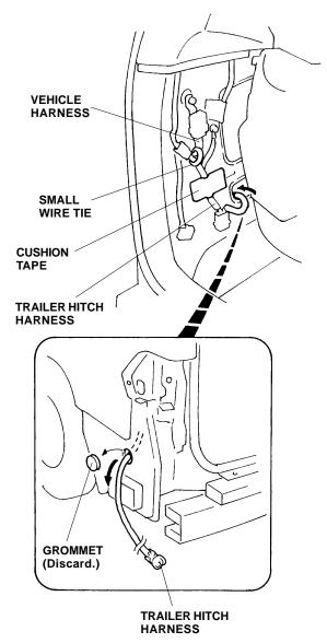
20. Remove and discard the grommet from the rear of the outside panel, and route the trailer harness out through the grommet hole.
