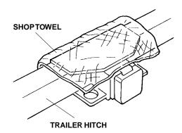
25. Secure the trailer harness to the back of the trailer hitch with one cushion tape.
