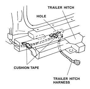
24. Place a shop towel over the trailer hitch. Route the trailer hitch harness through the hole in the bumper you drilled in step 7; then reinstall the rear bumper.
