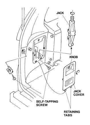
12. Remove the two self-tapping screws.
