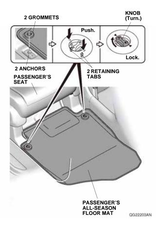
4. Insert the two tabs on the second row all-season floor mat under the two air vents. Place the grommets in the second row all-season floor mat over the anchors. Push the grommets into the anchors to secure the retaining tabs, then turn the knobs 90° to secure the second row all-season floor mat.
