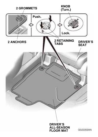
2. Place the grommets in the driver's all-season floor mat over the anchors. Push the grommets into the anchors to secure the retaining tabs, then turn the knobs 90° to secure the driver's all-season floor mat. 3. Place the grommets in the passenger's all-season floor mat over the anchors. Push the grommets into the anchors to secure the retaining tabs, then turn the knobs 90° to secure the passenger's all-season floor mat.
