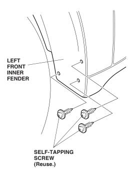
Position the left front splash guard on the left front inner fender. Attach the hook on the splash guard to the edge of the left side sill. Install the three self-tapping screws you removed. Tighten the three self-tapping screws in the order shown.
