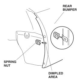
7. Position the left rear splash guard on the rear bumper and left rear inner fender, and install one self-tapping screw (short), one self-tapping screw (long) and one self-tapping screw removed in step 5. Tighten the three self-tapping screws in the order shown.
