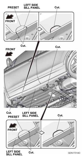
2. Remove the undercoating in the areas shown. Apply touch-up paint to the areas where you removed the undercoating, and allow them to dry thoroughly.
