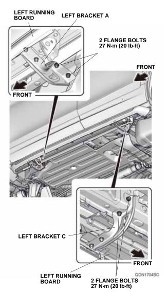
Tighten the four flange bolts loosely installed in step 3. Torque the flange bolts to 27 N·m (20 lb·ft).
