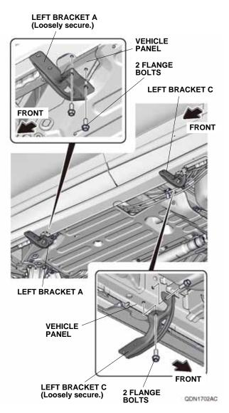
Secure the left running board to the left bracket A and left bracket C with four flange bolts. Torque the flange bolts to 27 N·m (20 lb·ft). NOTE: Have an assistant help you when installing the running board.
