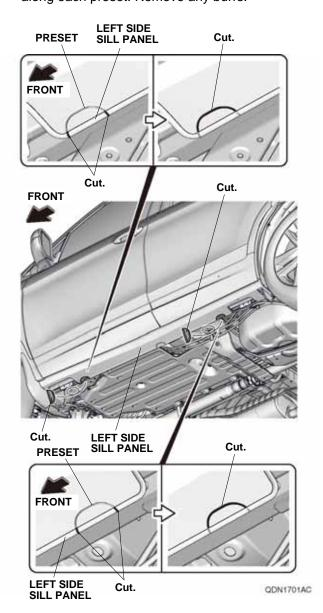
10. Remove the undercoating in the areas shown. Apply touch-up paint to the areas where you removed the undercoating, and allow them to dry thoroughly.
