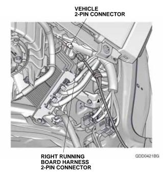
40. Secure the right running board harness to the vehicle harness with two wire ties.
