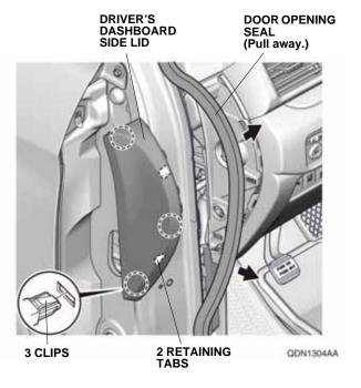
6. Remove the driver's dashboard lower cover, unplug the vehicle connectors, and release the vehicle sensor.
