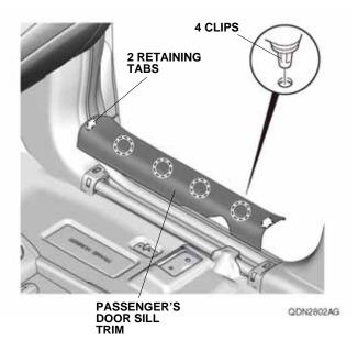
4. Pull away the door opening seal, and remove the passenger's kick panel.
