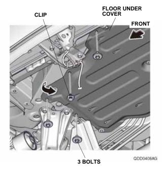
18. Remove the clip on the driver's side, and pull away the floor carpet.
