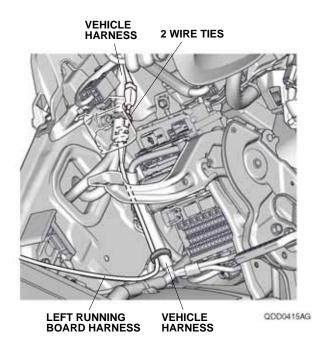
29. Secure the left running board harness to the vehicle harness with two wire ties.
