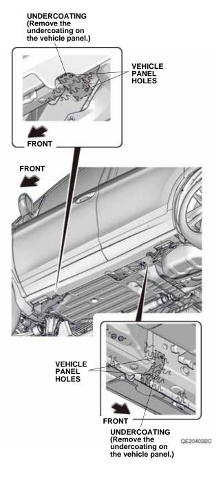
11. Loosely secure the left bracket A and left bracket C to the vehicle panel with four flange bolts.
