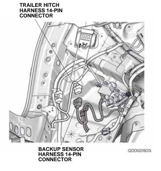
29. Install the 14-pin connectors to the trailer hitch harness 14-pin connectors as shown. Go to step 31.
