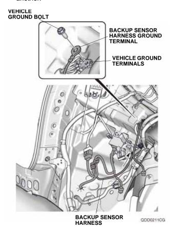
35. Secure the backup sensor harness to the vehicle harness with four wire ties.
