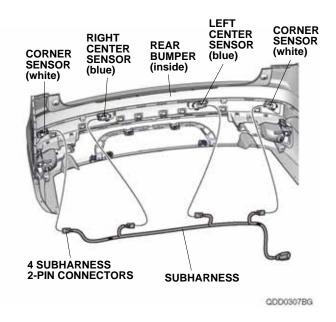
60. Line up and secure the green tape on the subharness to the rear bumper as shown.
