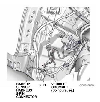
32. Secure the backup sensor harness grommet into the vehicle grommet hole.
