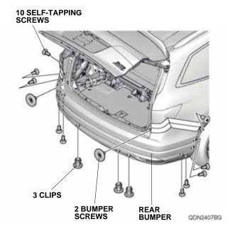
On each side, release the nine retaining tabs along the fenderwell.
