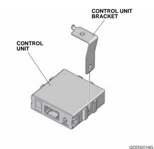
25. Insert the control unit bracket into the hole in the vehicle panel, and secure it with one flange bolt.
