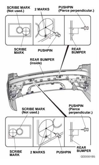
52. While wearing eye protection, drill the eight pierced marks with a 3 mm drill bit from the painted side of the rear bumper.
