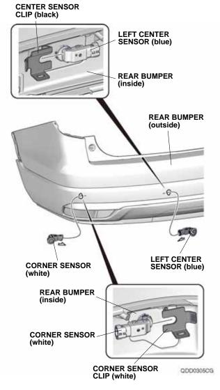
56. Secure the corner sensor (white) and left center sensor (blue) with corner sensor clip (white) and center sensor clip (black) as shown.
