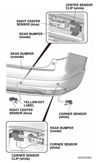
58. Secure the corner sensor (white) and right center sensor (blue) with corner sensor clip (white) and center sensor clip (white) as shown.
