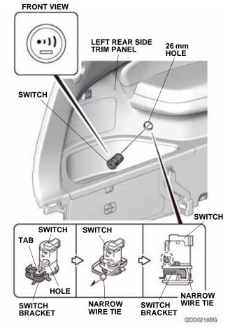
43. Line up the tab on the switch bracket with the hole in the switch and secure the switch bracket to the switch with one narrow wire tie.
