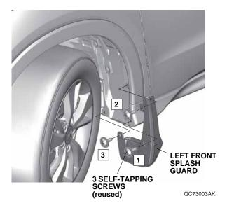
4. Remove the two self-tapping screws.
