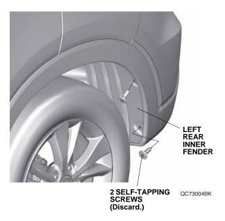
5. Install one spring nut on the left rear inner fender as shown.
