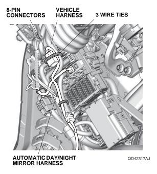
33. Route the automatic day/night mirror harness along the vehicle harness. Remove the bolt, and install the automatic day/night mirror harness ground terminal with one ground bolt.
