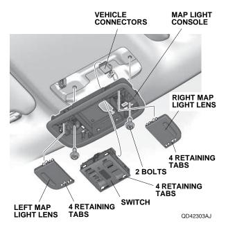
Without Moonroof: Remove the map light console and unplug the vehicle connector.
