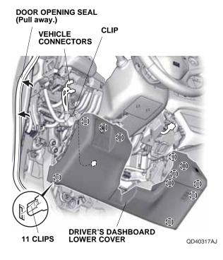
14. Pull away the door opening seal, and remove the driver's front door sill trim.
