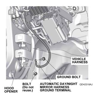
34. Secure the automatic day/night mirror harness to the vehicle harness with two wire ties.
