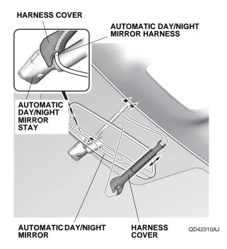
25. Route the automatic day/night mirror harness down the A-pillar as shown. Align the green tape on the automatic day/night mirror harness with the vehicle clip, and secure the automatic day/night mirror harness to the vehicle harness with two wire ties. Do not cover the installation holes of the driver's A-pillar trim.
