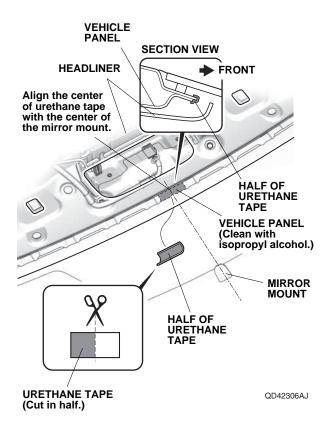
17. Using scissors, cut one urethane tape in half. Attach one half of urethane tape to the vehicle panel as shown. Be careful not to crease the headliner.
