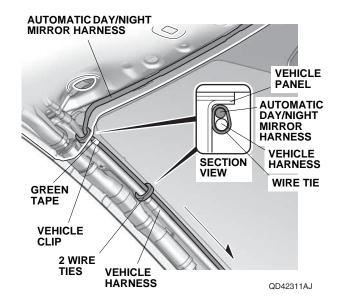
26. Align the green tape on the automatic day/night mirror harness with the vehicle clip, and secure the automatic day/night mirror harness to the vehicle harness with one wire tie.
