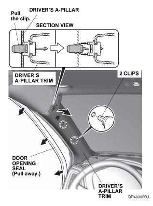
To prevent clips from falling into the body panel area, carefully insert a shop towel between the driver's A-pillar and the driver's A-pillar trim.
