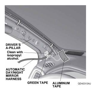
28. Line up the green tape on the automatic day/night mirror harness to the driver's A-pillar with one aluminum tape.
