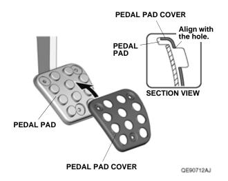
14. Using the hand riveter, install the pedal pad cover on the brake pedal with three rivets B in the order shown.
