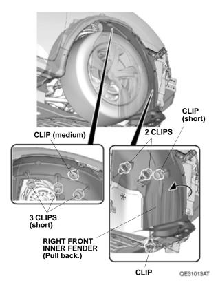
15. Remove the eight clips from the left front inner fender and pull it back as shown.
