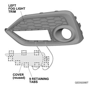
21. Install the left fog light trim to the front bumper with the 10 retaining tabs.
