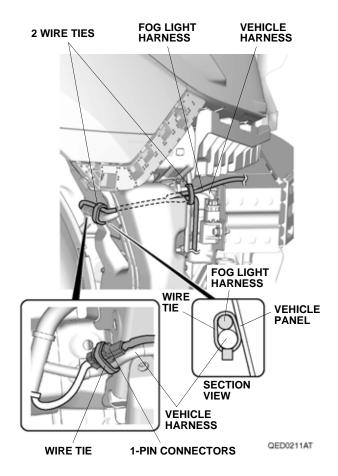
39. Route the fog light harness along the front bumper beam as shown.
