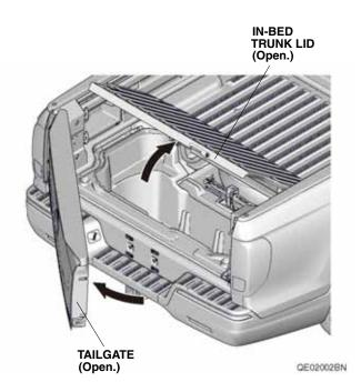
2. Remove the two holding bolts, pull back the tire tray, and rest it on the back edge of the in-bed trunk.
