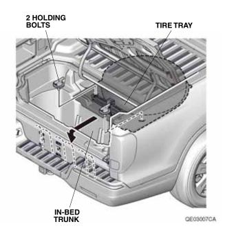
3. Store the towing kit in the tool box as shown. Install the tire tray.
