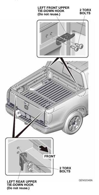
Install the left front bracket and left rear bracket to the left side bed lining with the four TORX bolts removed in step 1. Torque the TORX bolts to 20 N·m (15 lbf·ft). Repeat on the other side. NOTE: Make sure that the brackets are installed in the correct position and orientation.
