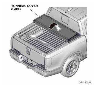
4. Tighten the wing nut of the tonneau cover and attach the clip to the left front bracket. Repeat on the other side.
