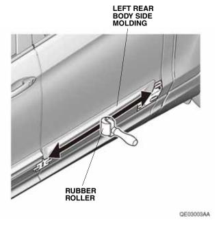
14. Remove the templates. Turn the templates over and repeat steps 1 through 13 to install the right body side moldings.
