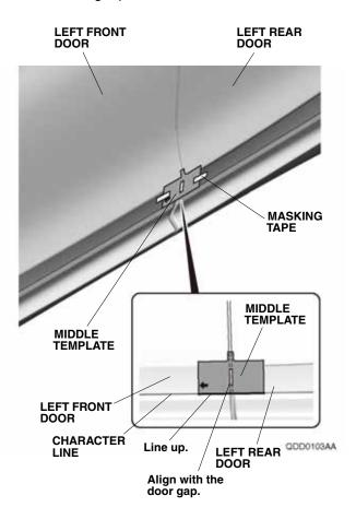
3. Fold the tab, line up the rear template with the character lines and attach it to the left rear door with masking tape as shown.
