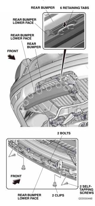
5. Remove the two clip nuts from the rear bumper lower face, and install them on the trailer hitch cover.
