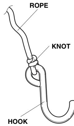
10. Route the other end of the rope through the bottom of the ratchet hook in the direction shown, and turn the spool until the rope end comes out of the ratchet.
