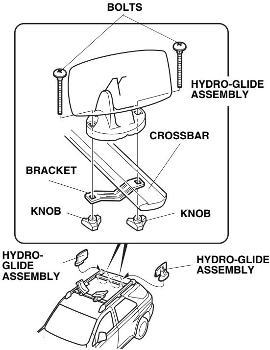
3. Rest the front of the kayak on the hydro-glide assemblies. Standing beside or alongside the kayak, lift up the rear portion of the kayak and push it forward, sliding on the hydro-glide assemblies and saddles. Make sure the kayak reaches the front saddles before you lower it.
