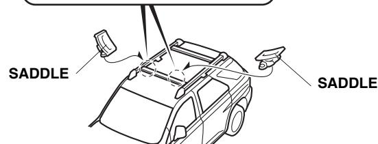
2. Position the two hydro-glide assemblies on the rear crossbar. Loosely install the hydro-glide assemblies with one bracket, two bolts, and two knobs for each assembly. The distance between the two assemblies should be the same width as the kayak.
