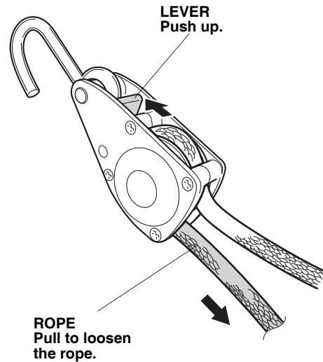
12. Attach one ratchet hook to the front attachment strap, and one ratchet hook to the rear attachment strap. Attach the front hook to the front bumper beam or tow hook. Attach the rear hook to the rear bumper beam or the trailer hitch. Secure the kayak to the vehicle by pulling the rope through the ratchet hooks.
