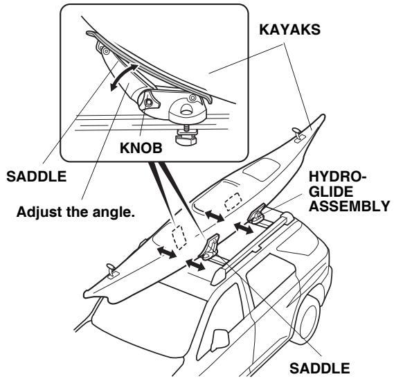
5. Slide the kayak forward and backward until it's level with the roof. If necessary, loosen the knob of each saddle and adjust the saddle angle to fit snugly against the kayak. Tighten each knob securely.
