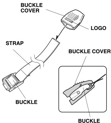
7. Route the strap under the front crossbar, and around the kayak as shown. Slide the buckle cover away from the buckle, route the strap through the buckle, and tighten the strap. Slide the buckle cover back over the buckle.
