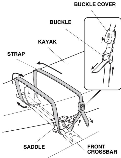
8. Route the strap under the rear crossbar, and around the kayak as shown. Slide the buckle cover away from the buckle, route the strap through the buckle, and tighten the strap. Slide the buckle cover back over the buckle.
