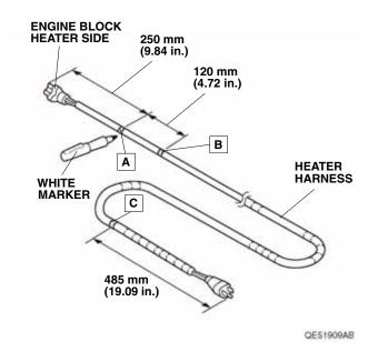
12. Install one wire tie with clip to the heater harness at point A.
