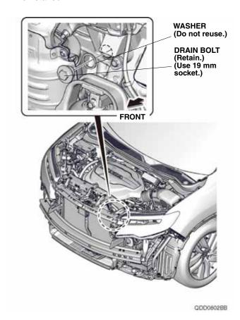
Install the engine block heater with the aluminum washer into the bolt hole using a 24 mm socket.
