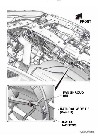
18. Route the heater harness along the fan shroud, and secure the heater harness to the fan shroud ribs with two natural wire ties and one black wire tie.
