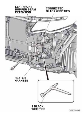
22. Bundle up the excess heater harness, and secure the heater harness with two black wire ties.
