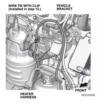
17. Route the heater harness toward the fan shroud, and secure the heater harness to the fan shroud rib with one natural wire tie at point B.
