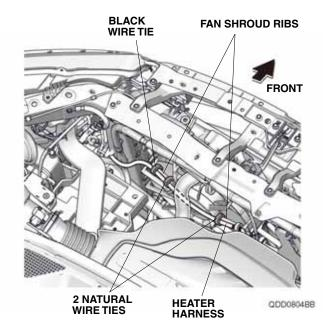
19. Route the heater harness through the front bulkhead, and secure the heater harness to the vehicle harness with three black wire ties.
