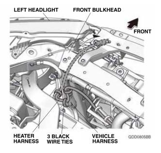
20. Route the heater harness down under the front bumper beam, and secure the heater harness to the left front air guide plate with one black wire tie at the point C.
