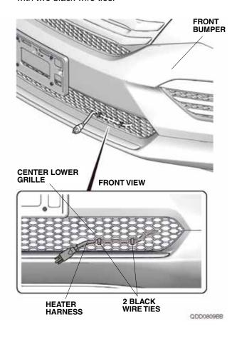
26. Attach the protective cap to the center lower grille, and plug the heater harness connector into the protective cap.
