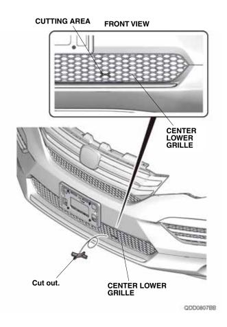
24. With the help of an assistant, bring the front bumper close to the vehicle. Route the heater harness through cutout on the center lower grille, then install the front bumper.
