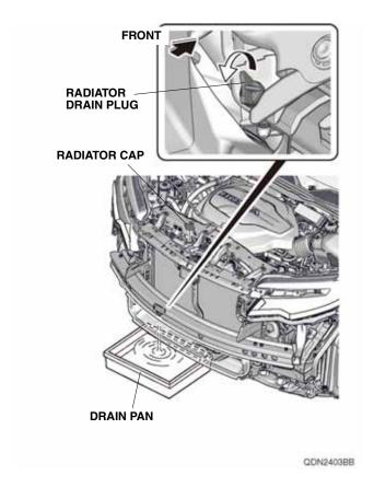
10. Drain the coolant completely, then reinstall the radiator cap.
