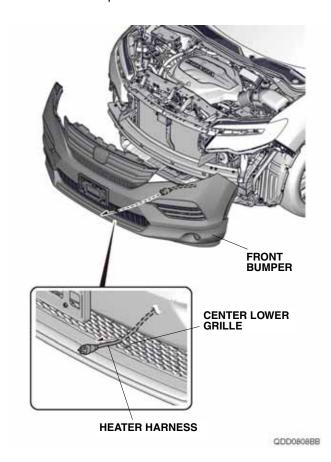
25. Secure the heater harness to the center lower grille with two black wire ties.
