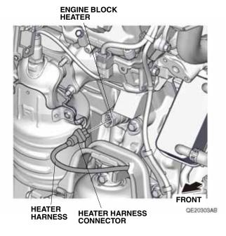
16. Route the heater harness in the direction shown, and secure the heater harness to the vehicle bracket with one wire tie with clip installed in step 12.
