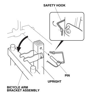
2. Install the pin and safety hook as shown.
