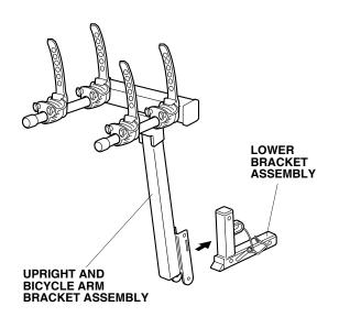
2. Install the 8 x 70 mm bolt, two 8 mm washers, and 8 mm nut as shown. Tighten the bolt securely.
