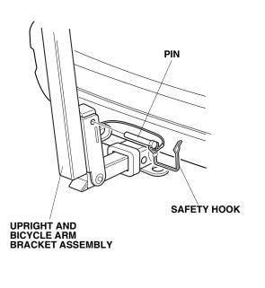
2. Gently lower the upright and bicycle arm bracket assembly to the stop position.
