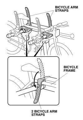
4. Install the two anti-sway straps and tighten each anti-sway strap securely around the bicycle frame.
