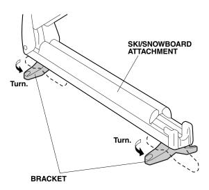
4. Using the wrench supplied, install the ski/snowboard attachment to the front crossbar with four bolts, four collars, and two brackets.
