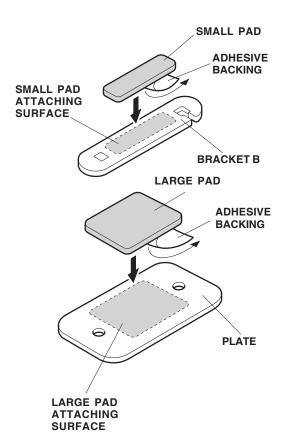
3. Using isopropyl alcohol on a shop towel, clean four plates where the large pads will attach. Remove the adhesive backings from the large pads and attach them to the plates.
