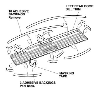
19. Remove the remaining adhesive backings.
