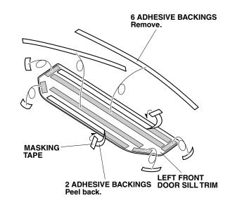
8. Remove the remaining adhesive backings.
