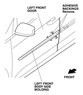
Using a rubber roller, apply pressure against the left front body side molding and roll from one end to the other.
