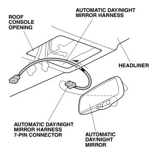
8. Align the green tape on the automatic day/night mirror harness to the edge of the headliner.
