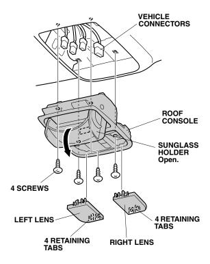
4. Rotate each sunvisor holder 45° counterclockwise, then remove it.
