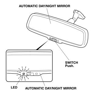
2. Push the switch. Check that the LED illuminates.
