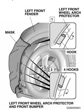
3. Attach four hooks on the mask's bumper section to the edge of the left front wheel arch protector and front bumper.
