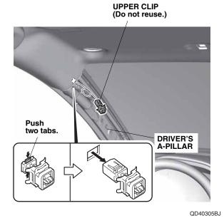
10. Install the new clip (supplied) to the driver's A-pillar trim.Go to step 12.
