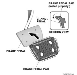
9. Loosely install the brake pedal pad cover on the brake pedal pad.
