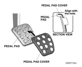
14. Using the hand riveter, install the pedal pad cover on the brake pedal with three rivets B in the order shown.
