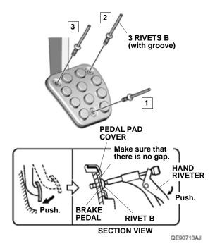
15. Repeat steps 11 through 14 to install the pedal pad and pedal pad cover on the clutch pedal.
