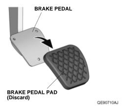
12. Install the pedal pad on the brake pedal.
