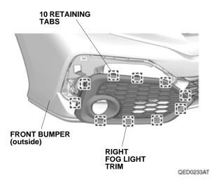
27. Install the right fog light trim to the front bumper with one clip. Go to step 34.
