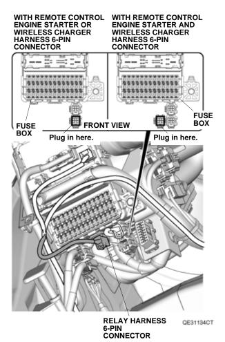
57. Secure the relay harness to the vehicle harness with five wire ties.
