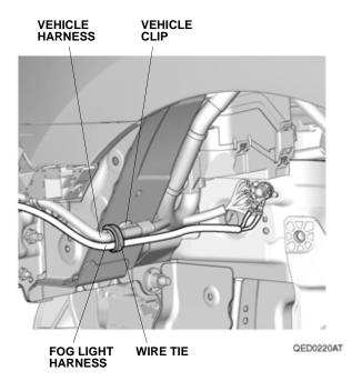
48. Plug two fog light harness 2-pin connectors into each fog light, then with the help of an assistant, install the front bumper.
