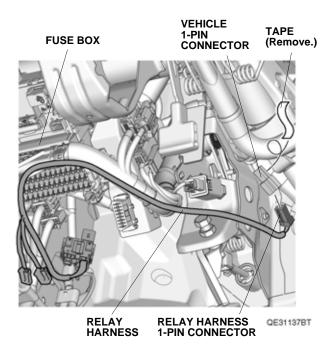
52. Route the relay harness as shown. Attach the wire tie with holder to the relay harness relay block and secure it to the vehicle harness with the wire tie with holder.
