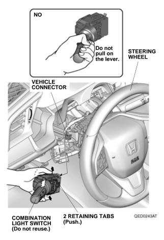
61. While pushing the two retaining tabs, slide the combination light switch out and remove it from the steering column.
