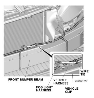
45. Line up the fog light harness with the vehicle clip and secure the fog light harness to the vehicle harness with one wire tie.
