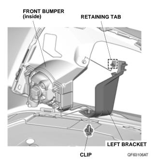
31. Install the left fog light trim to the front bumper with the 10 retaining tabs.
