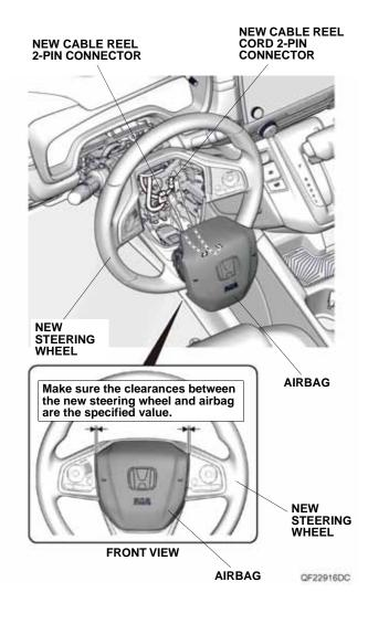
58. Check clearance around the heater harness while moving the new steering wheel up and down, back and forth.
