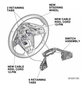
51. Install the control unit on the steering wheel trim.
