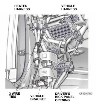
34. Route the heater harness along the vehicle harness, and secure it to the vehicle harness with two wire ties.
