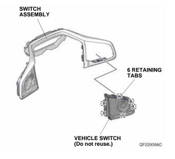
49. Install the HSW switch on the switch assembly.
