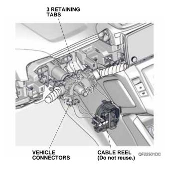
28. Remove the locking pin. Install the new cable reel with three retaining tabs, and plug the vehicle connectors into the new cable reel.
