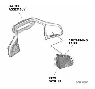
50. Plug two new cable reel cord 12-pin connectors into the switch assembly, and install the switch assembly on the new steering wheel.
