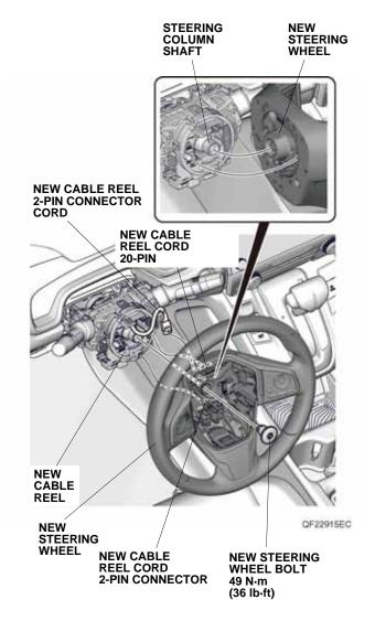
56. Install the new steering wheel bolt. Torque the new steering wheel bolt to 49 N·m (36 lb·ft). Tighten to the specified torque within 5 minutes.
