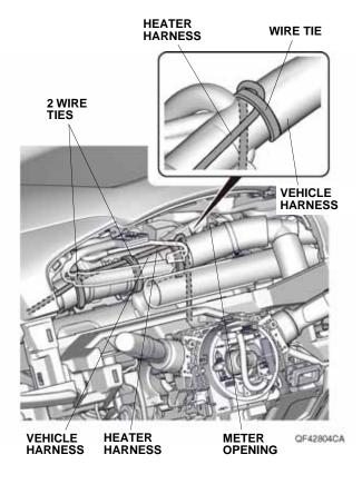
40. Secure the heater harness to the vehicle harnesses with two wire ties.
