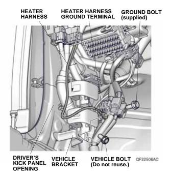
33. Secure the heater harness to the vehicle bracket and vehicle harness with three wire ties.
