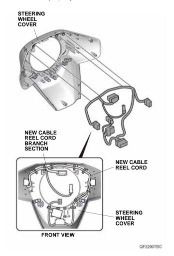
47. Plug the new cable reel cord 4-pin connector into the new steering wheel 4-pin connector, and install the steering wheel cover on the new steering wheel.
