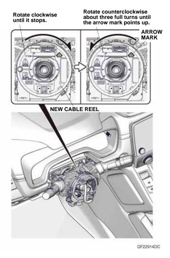
54. Before installing the new steering wheel, make sure the front wheels are still pointing straight-ahead. To confirm the cable reel is line up properly, rotate the cable reel clockwise until it stops, then rotate it counterclockwise about three full turns. The arrow mark on the cable reel label must point straight up.
