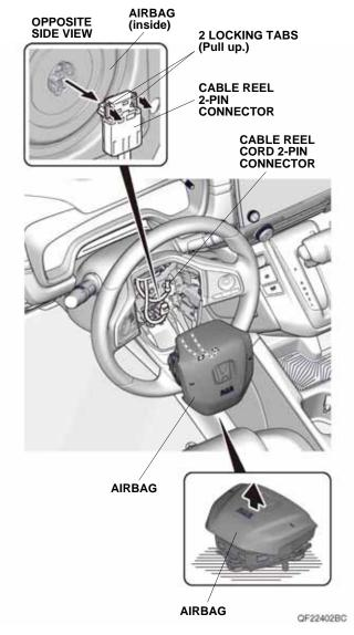
Remove the airbag. Do not drop the removed airbag or hit it on an object. Place the removed airbag in a safe place with the padded surface (top) facing up. 11. With the front wheels line up in the straight-ahead position, unplug the vehicle connector from the cable reel, and loosen the steering wheel bolt.
