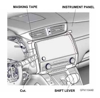
22. Remove the climate control unit and unplug the vehicle connector.
