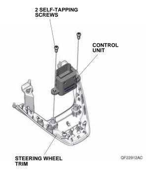
52. Plug the new cable reel cord 14-pin connector into the control unit, and install the steering wheel trim on the new steering wheel with two self-tapping screws removed in step 42.
