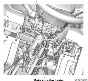
Make sure the heater harness does not interfere with the vehicle.
