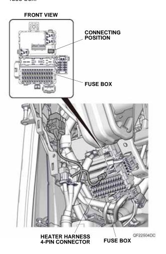
32. Remove the vehicle bolt. Route the heater harness as shown, and secure the heater harness ground terminal to the vehicle bracket with the ground bolt.
