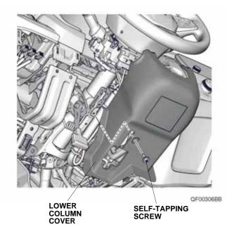
62. Connect the negative cable to the battery, then turn the engine switch to ON. Turn the steering wheel 90° clockwise. Secure the lower column cover.
