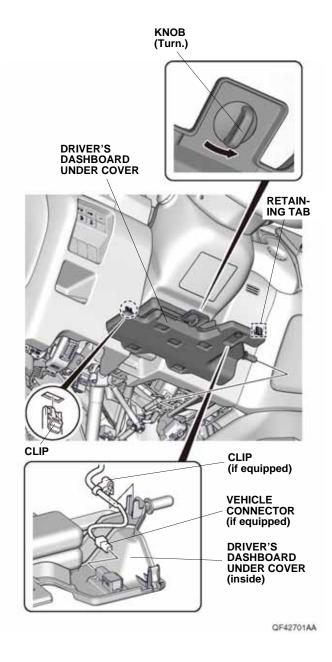
4. Remove the driver's dashboard lower cover and unplug the vehicle connectors.
