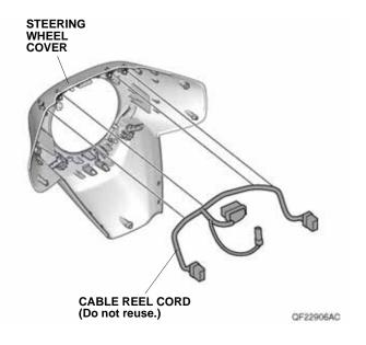
46. Install the new cable reel cord on the steering wheel cover.
