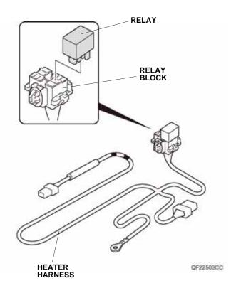
30. Attach the relay block on the heater harness to the vehicle panel.
