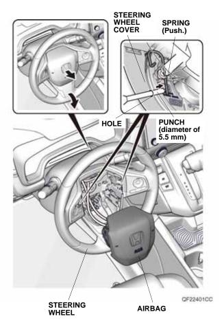
8. Insert a punch (diameter of 5.5 mm) through the left hole of the steering wheel cover, and push the spring to release the airbag. Repeat for the other side.
