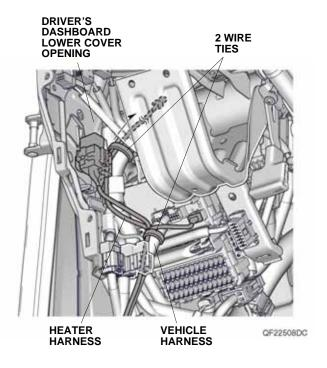
35. Route the heater harness along the vehicle harness, and secure it to the vehicle harness with two wire ties.
