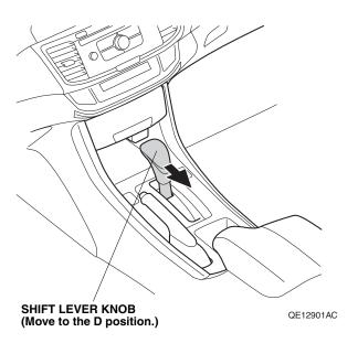
15. Attach tape to the shift lever knob and center console panel as shown.
