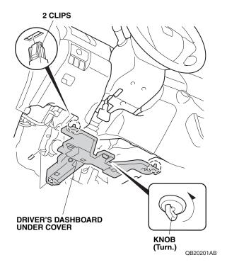
3. Remove the driver's dashboard lower cover and unplug the vehicle connectors.
