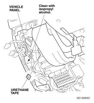
27. Attach the urethane tape to the vehicle panel as shown.
