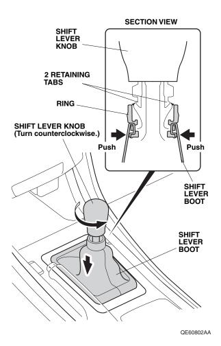
11. Remove the shift lever knob. Go to step 16.
