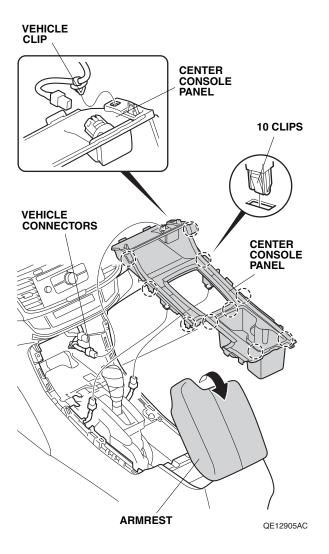
20. Remove the vehicle lower tray from the center console panel.
