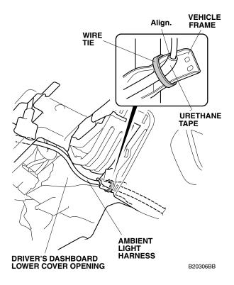
18. Secure the ambient light harness to the vehicle harness with one wire tie. Move the steering wheel up and down through its full adjustment range and make sure the harness is not being stretched.
