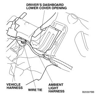
19. On the passenger's side of the vehicle, route and secure the ambient light harness to the vehicle harness with two wire ties.
