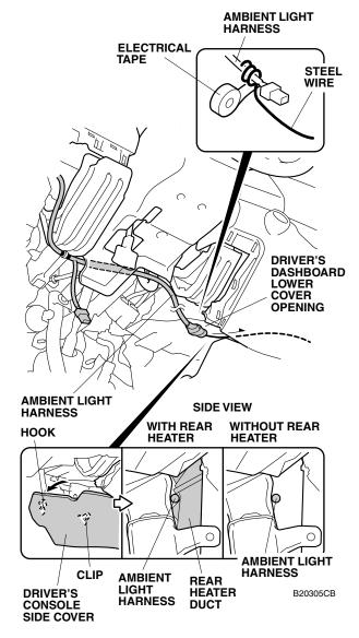
14. Attach a piece of steel wire to the ambient light harness with electrical tape. Route the ambient light harness through the center console from the driver's dashboard lower cover opening to the passenger's under cover opening. Release the passenger's console side cover.
