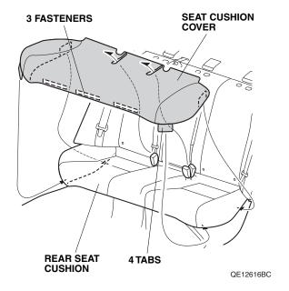
19. Insert the seat cushion cover between the rear seat back and the rear seat cushion, and secure the three fasteners to the rear seat cushion.
