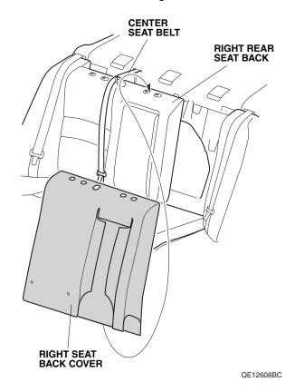
10. Secure the fastener on the right rear seat back. Raise the right rear seat back and lock it to its original position.
