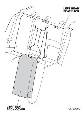
12. Secure the fastener on the left rear seat back. Raise the left rear seat back and lock it to its original position.
