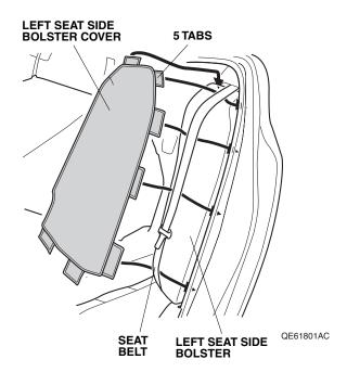
6. Secure the three fasteners to the left seat side bolster.
