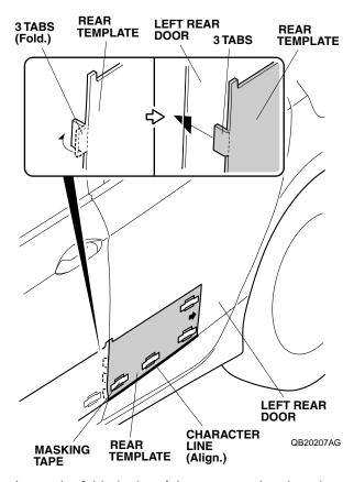
4. Insert the folded tabs of the rear template into the opening between the rear door and the B-pillar. Align the template with the character line, and tape the template to the door with strips of masking tape.
