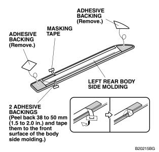
13. Align the left rear body side molding with the rear template, and attach it to the left rear door as shown.
