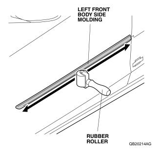
12. Peel back approximately 38 to 50 mm (1.5 to 2.0 in.) of adhesive backing from each adhesive strip, and tape the ends to the front surface of the body side molding. Remove the small end pieces of the adhesive backing.
