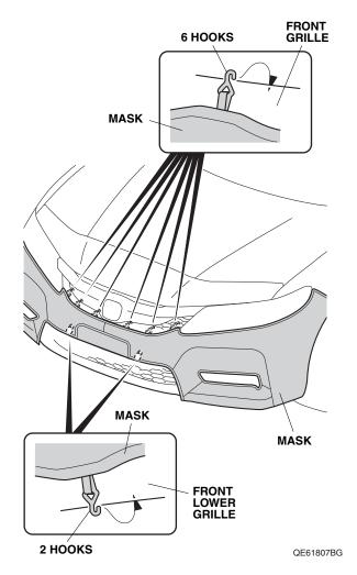
11. Attach two hooks to the inside edge of the front lower grille.
