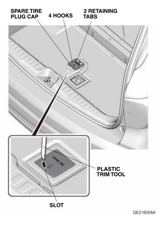
3. Remove the spare tire plug to access the spare tire hoist shaft. Lower the spare tire completely.
