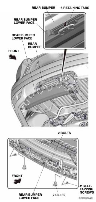
5. Remove the two clip nuts from the rear bumper lower face, and install them on the trailer hitch cover.
