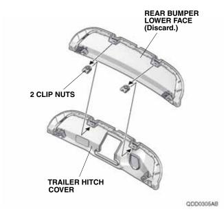
6. Install the trailer hitch cover to the rear bumper with six retaining tabs, two clips, two self-tapping screws, and two bolts removed in step 4.
