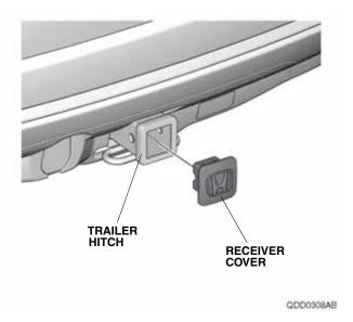
Install the ball mount into the trailer hitch using a hitch pin clip and hitch pin. And store the receiver cover in the cargo area
