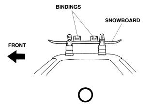
11. If the bindings cannot be positioned between the front and the rear attachments, install the rear binding behind the rear attachment as shown.
