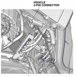
RIGHT RUNNING BOARD HARNESS 2-PIN CONNECTOR QDD0421BG
