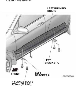
Tighten the four flange bolts loosely installed in step 11. Torque the flange bolts to 27 N·m (20 lbf·ft).
