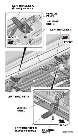
Secure the left running board to the left bracket A and left bracket C with four flange bolts. Torque the flange bolts to 27 N·m (20 lbf·ft). NOTE: Have an assistant help you when installing the running board.
