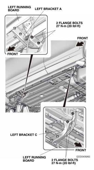
14. Align the green tape on the left running board harness with the hole on the left bracket A, and secure the left running board harness to the left bracket A with one wire tie.
