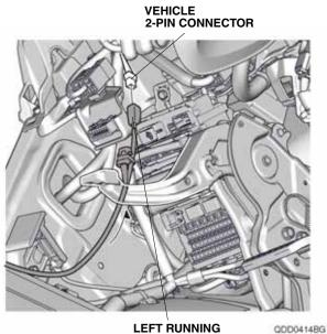
LEFT RUNNING CODO41 BOARD HARNESS 2-PIN CONNECTOR 28. Secure the left running board harness to the vehicle harness with two wire ties.
