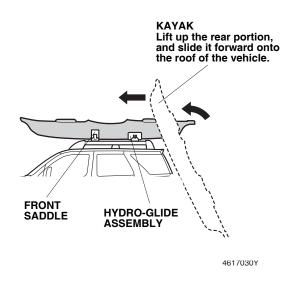
4. Adjust the distance of the saddles and hydro-glide assemblies to the same width as the kayak, then secure the saddles and the hydro-glide assemblies by tightening the knobs you installed in steps 1 and 2.
