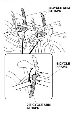
4. Install the two anti-sway straps and tighten each anti-sway strap securely around the bicycle frame.
