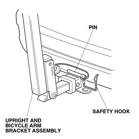
2. Gently lower the upright and bicycle arm bracket assembly to the stop position.
