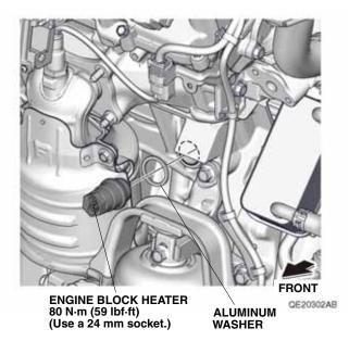
15. Plug the heater harness connector into the engine block heater. Make sure the heater harness connector is fully seated in the engine block heater.
