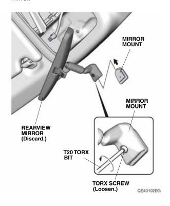
4. Install the automatic day/night mirror on the mirror mount as shown, and tighten the TORX screw.
