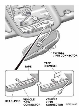
6. Route the vehicle harness as shown, and plug the vehicle 7-pin connector into the automatic day/night mirror. Be careful not to crease the headliner.
