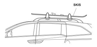
If the bindings cannot be positioned between the front and the rear attachments, install the skis with the rear bindings behind the rear attachment as shown.
