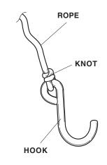
10. Route the other end of the rope through the bottom of the ratchet hook in the direction shown, and turn the spool until the rope end comes out of the rachet.
