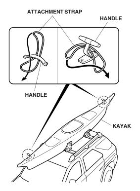
12. Attach one ratchet hook to the front attachment strap, and one ratchet hook to the rear attachment strap. Attach the front hook to the front bumper beam or tow hook. Attach the rear hook to the rear bumper beam or the trailer hitch. Secure the kayak to the vehicle by pulling the ropes through the ratchet hooks.
