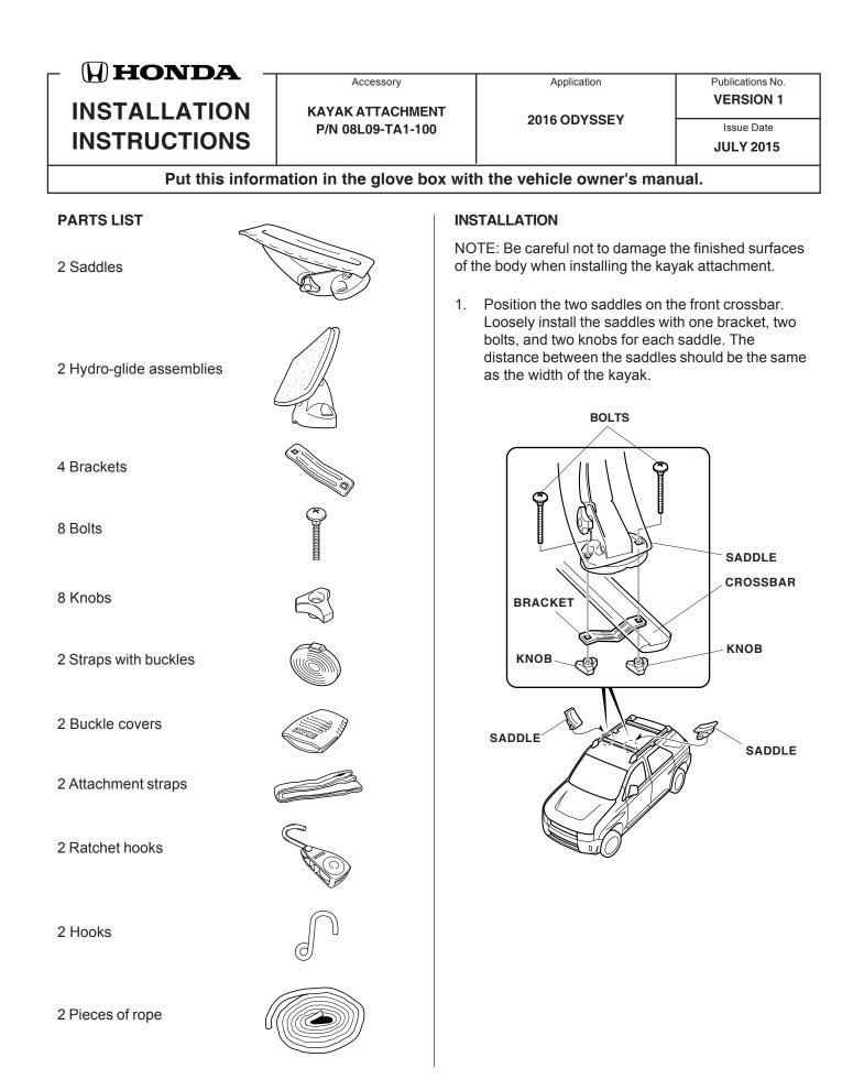
2. Position the two hydro-glide assemblies on the rear crossbar. Loosely install the hydro-glide assemblies with one bracket, two bolts, and two knobs for each assembly. The distance between the two assemblies should be the same as the width of the kayak.
