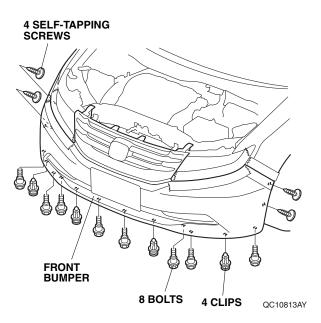
• On each side, release eight retaining tabs from the front bumper.
