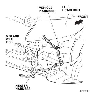
25. Route the heater harness down under the left headlight and forward. Secure the heater harness to the vehicle harness with one black wire tie.
