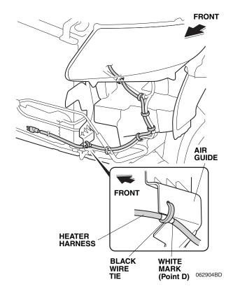
28. With the help of an assistant, route the heater harness through the front bumper in the area shown, and reinstall the front bumper.
