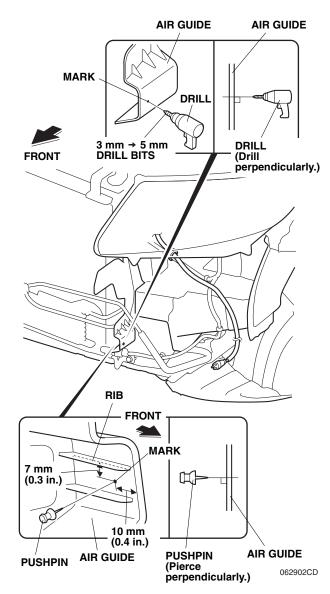
22. While wearing an eye protection, drill the pierced point with a 3 mm drill bit and widen the hole with a 5 mm drill. Remove any burrs.
