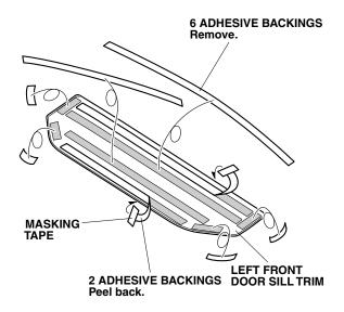
8. Remove the remaining adhesive backings.
