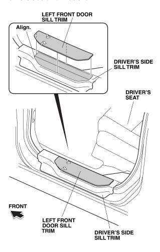
While applying light pressure against the left front door sill trim, carefully remove the two adhesive backings.
