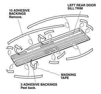
19. Remove the remaining adhesive backings.
