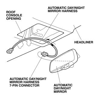
8. Align the green tape on the automatic day/night mirror harness to the edge of the headliner.
