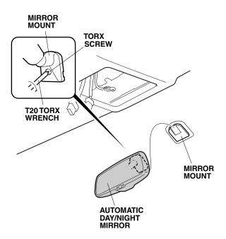
7. Route the automatic day/night mirror harness as shown. Plug the automatic day/night mirror harness 7-pin connector to the automatic day/night mirror.
