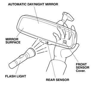
4. With the parking brake applied, step on the brake pedal and move the select lever to the "R" position. Repeat step 3, and make sure that the mirror surface does not dim. If the automatic day/night mirror does not function properly, check the fuse and all connectors.
