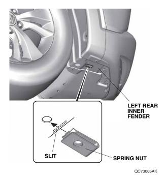
6. Secure the left rear splash guard with two 5 x 25 mm self-tapping screws and one 5 x 18 mm self-tapping screw in the order shown below.
