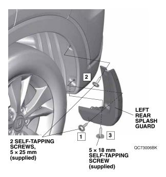
7. Turn the steering wheel fully clockwise, and repeat steps 2 through 6 to install the right splash guards.
