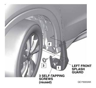
4. Remove the two self-tapping screws.
