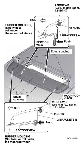
13. Tighten two screws and two nuts on the front of the vehicle first, then tighten two screws and two nuts on each side. Tighten while applying pressure so that there is no gap between the roof panel and the brackets A and B. Torque the screws to 2.0 N·m (1.5 lbf·ft).
