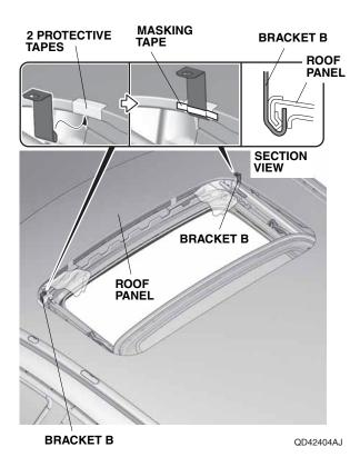
9. Place two brackets A into position over the two protective tapes and around the lip of the roof panel, and tape them into position with the strips of masking tape. Be sure to align the lower end of the brackets A with the second indentation.
