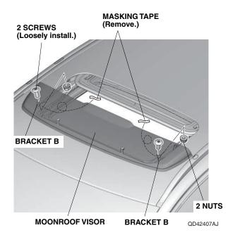
Position the moonroof visor with equal spacing in the front and on the sides. Check that the rubber molding is not twisted or rolled under the moonroof visor.
