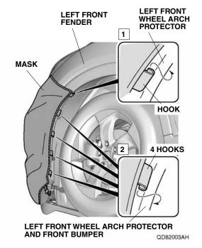
3. Attach four hooks on the mask's bumper section to the edge of the left front wheel arch protector and front bumper.
