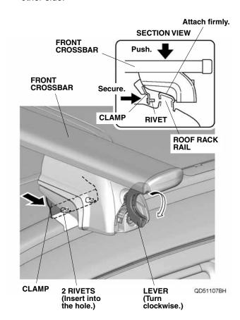
15. Lower the lever, and lock with key. Repeat on the other side.
