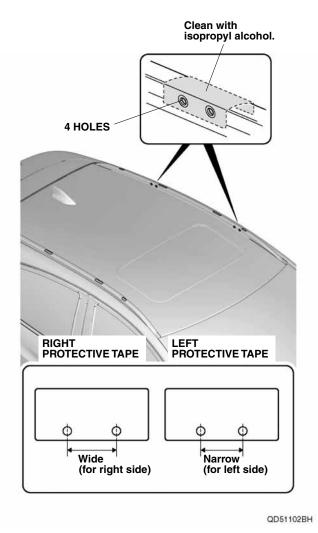
3. Align the left protective tape on the left roof rack rail, and attach masking tape to the left roof rack rail as shown.
